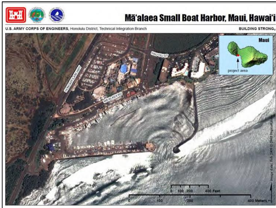
Figure 5. Maalaea Harbor 2009 air view with jetty configurations and southerly approaching wave patterns (USACE 2011). Note wave action covering eastern half of harbor made unsuitable for moorage and berthing. Breakers along west jetties and reef to east show shoreline, surf zone, and related sediment transport moved offshore.
